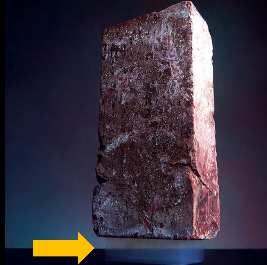
A 2.5 kg brick supported by a piece of aerogel with a mass of 2 grams
