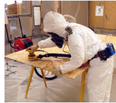
Worker with full protective gear conducting CPWR test inside a special chamber using a dust collection system
