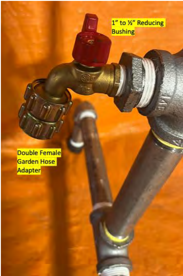
Pipe Stand Patch and Valves
