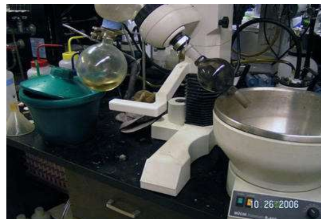
The lower round-bottomed flask from the rotovap exploded inside the metal water bath
