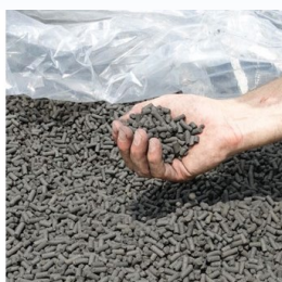
Application of bioamended SediMite™ that combines the advantages of adsorption by activated carbon and degradation by microbes for in situ cleanup of PCB-contaminated sediments.
