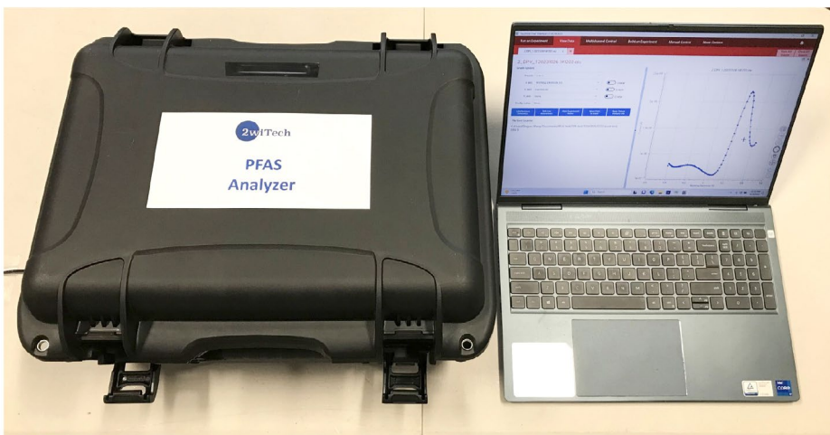
A portable PFAS analyzer (left) and its laptop-based controller (right). The PFAS analyzer comprises an electrochemical workstation, a testing module, and a solution delivery module.
