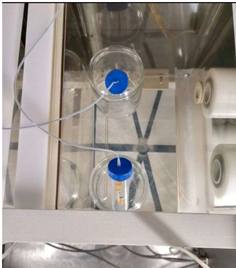
Figure A-69. Measurement Setup with Nano-T Sensor in Mouse Phantom
