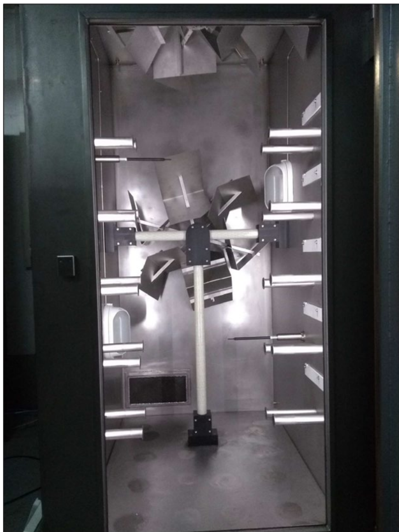
Figure A-1. Internal View of a Reverberation Chamber
