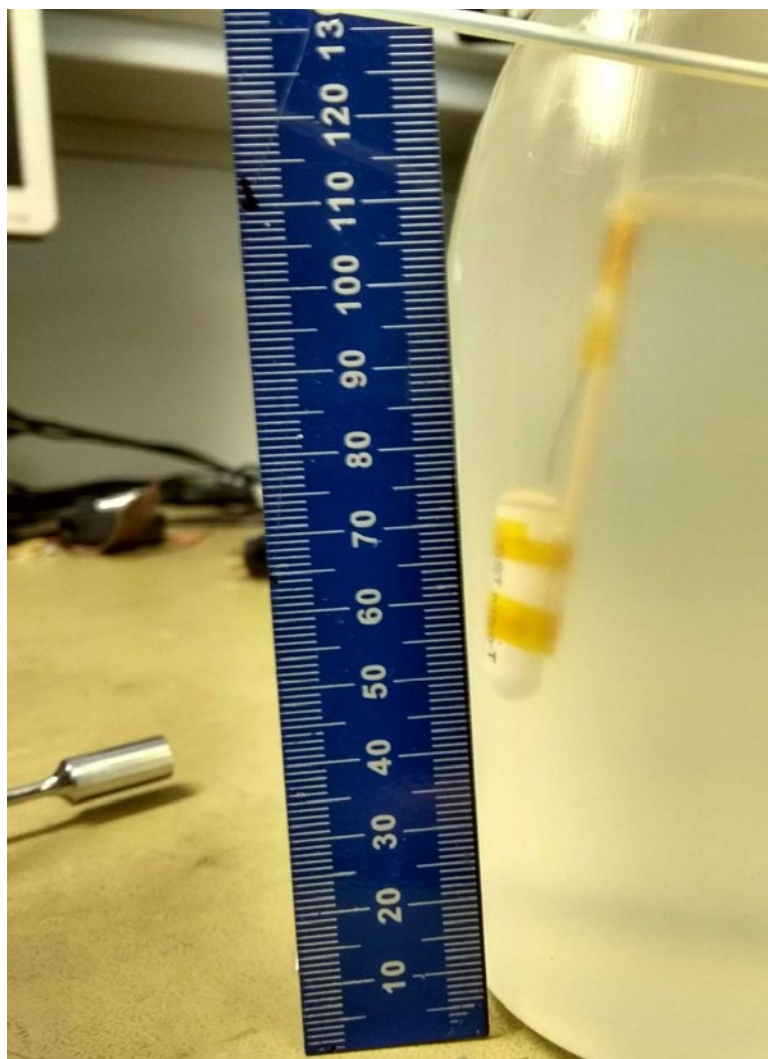
Figure A-67. Placement of the Implantable Micro-T Sensor within the Rat Phantom
