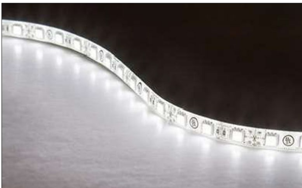
Figure A-13. (A) Light Emitting Diode Corner Profile and (B) Typical Waterproof Lighting Strip
