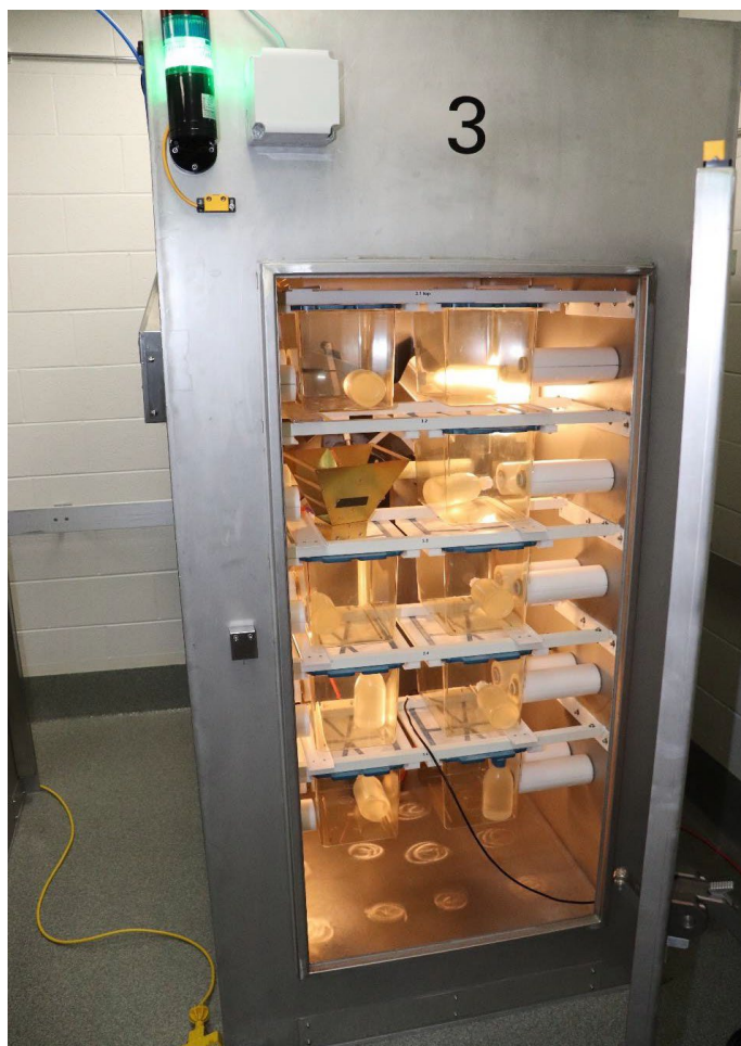
Figure B-1. One of the Reverberation Test Chambers at the Testing Facility
