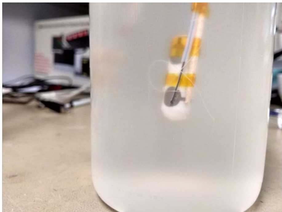
Figure A-68. Placement of the Implantable Micro-HRT Sensor within the Rat Phantom
