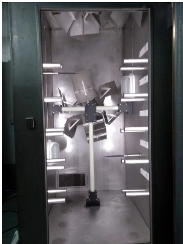
Figure 1. Internal View of a Reverberation Chamber
