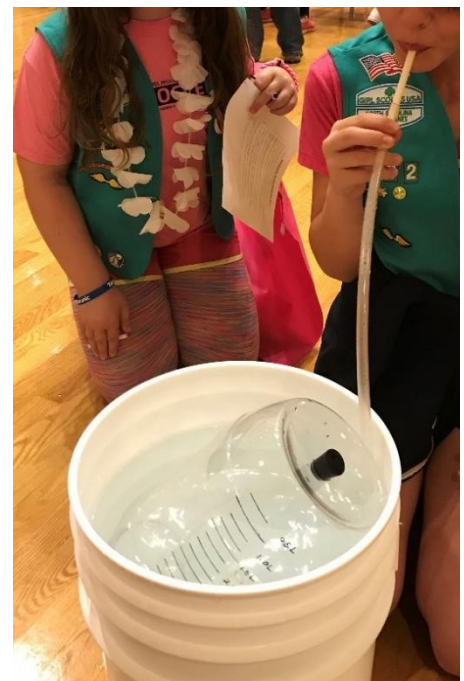
FVC Estimator in action, showing the bucket, plastic container and a volunteer blowing into the tube.
